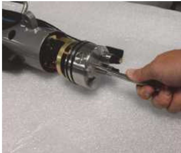
Figure 4-11: Pulling the Electronics Chassis out of the Towfish Housing
