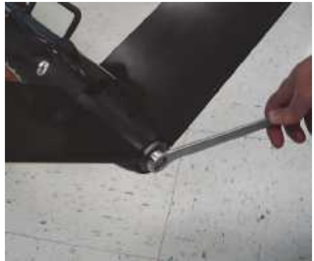
Figure 4-1: Loosening the Tail Cone Retaining Bolt
