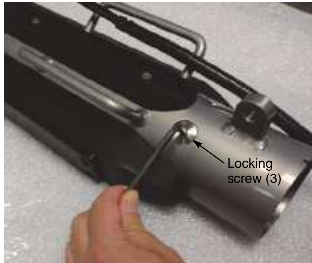
Figure 4-10: Tightening the Locking Screws in the Towfish Housing Aft End Cap
