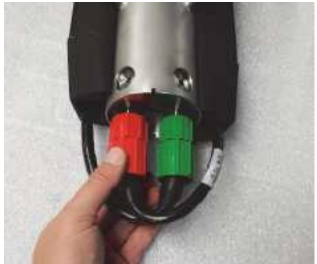
Figure 4-5: Disconnecting the Transducer Cables
