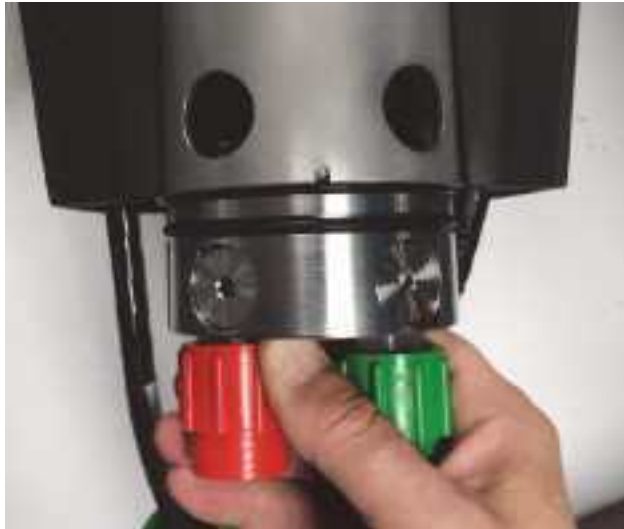
Figure 4-13: Aligning the Locking Screws before Inserting the Forward End Cap
