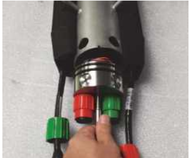
Figure 4-8: Pulling the Forward End Cap out of the Towfish Housing
