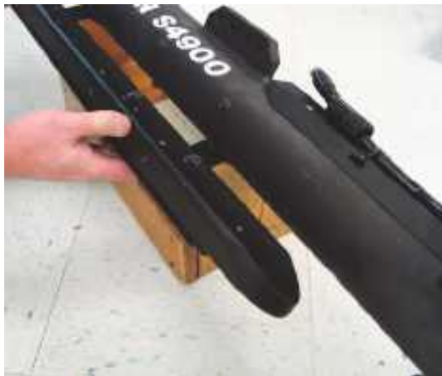
Figure 4-16: Separating a Transducer Assembly from the Towfish Housing
