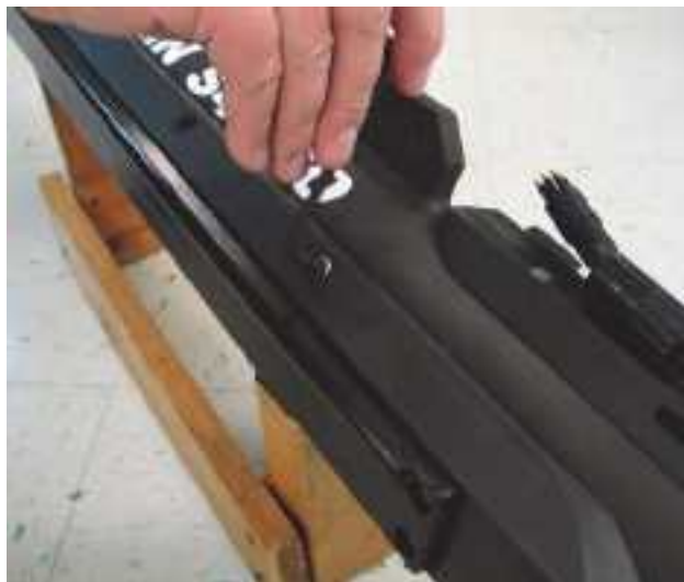
Figure 4-15: Removing the Eight Socket Head Cap Screws Securing a Transducer Assembly
