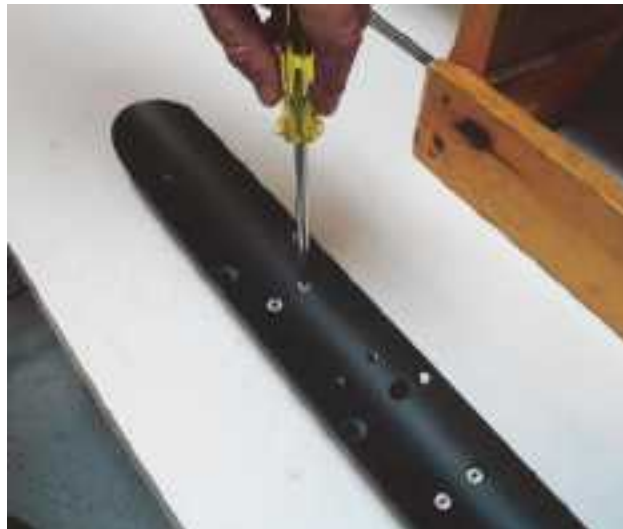
Figure 4-18: Removing the Eight Phillips Head Screws Securing the Transducer
