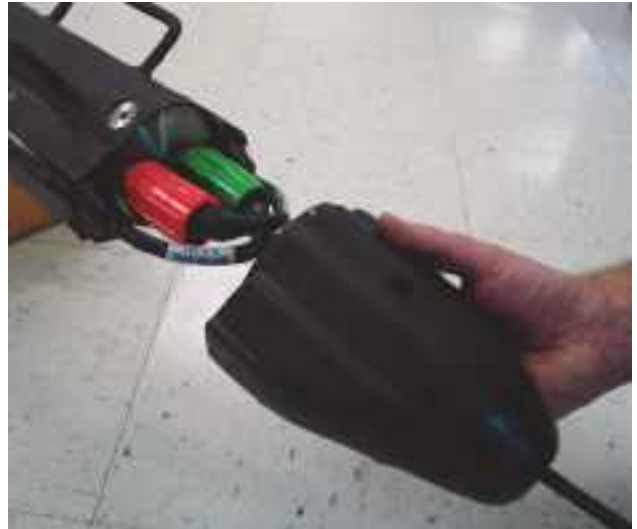
Figure 4-4: Removing the Nose Cone
