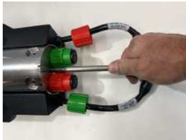
Figure 4-7: Screwing the Tail Cone Retaining Bolt into the Forward End Cap
