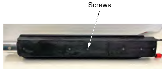
Figure 4-15: Removing the Phillips Head Screws Securing the Skidplate
