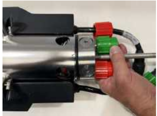
Figure 4-8: Pulling the Forward End Cap out of the Towfish Housing
