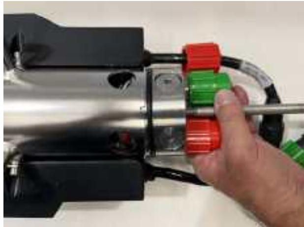
Figure 4-13: Aligning the Locking Screws before Inserting the Forward End Cap
