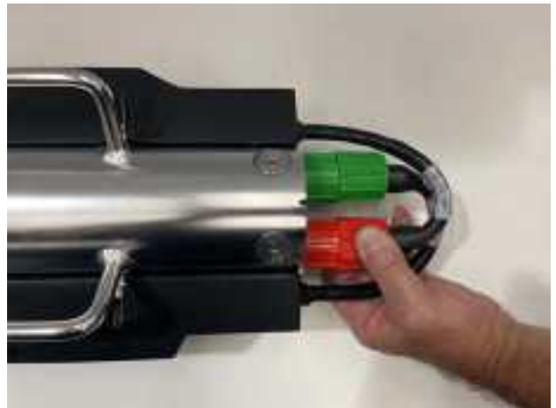
Figure 4-5: Disconnecting the Transducer Cables
