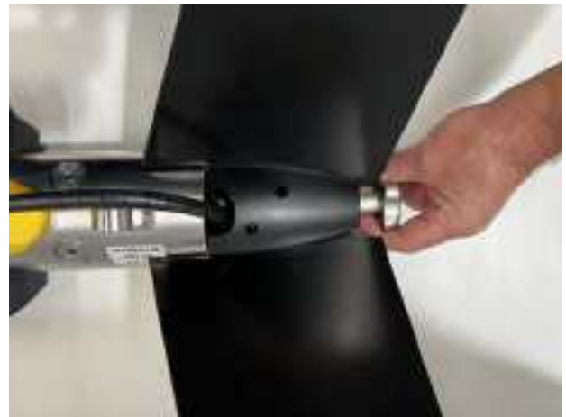
Figure 4-1: Loosening the Tail Cone Retaining Bolt
