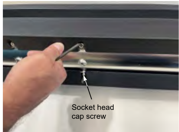
Figure 4-17: Removing of the Ten Socket Head Cap Screws of a Transducer
