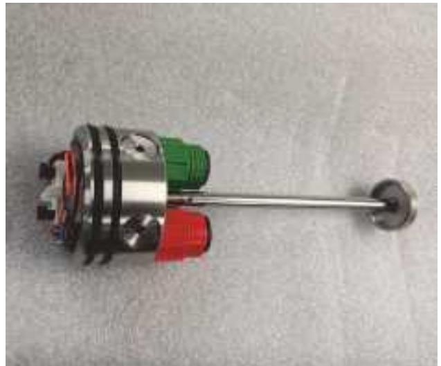
Figure 4-9: Forward End Cap Removed from the Towfish Housing
