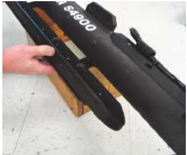
Figure 4-16: Separating a Transducer Assembly from the Towfish Housing
