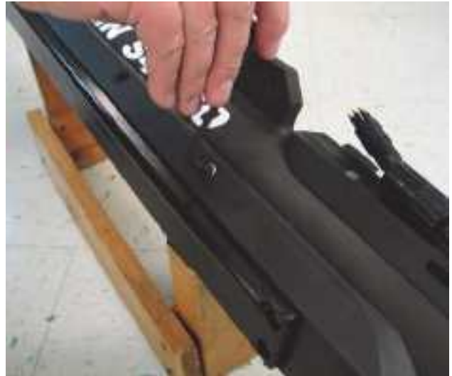
Figure 4-15: Removing the Eight Socket Head Cap Screws Securing a Transducer Assembly
