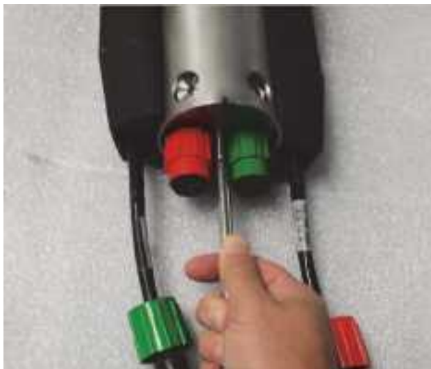
Figure 4-7: Screwing the Tail Cone Retaining Bolt into the Forward End Cap
