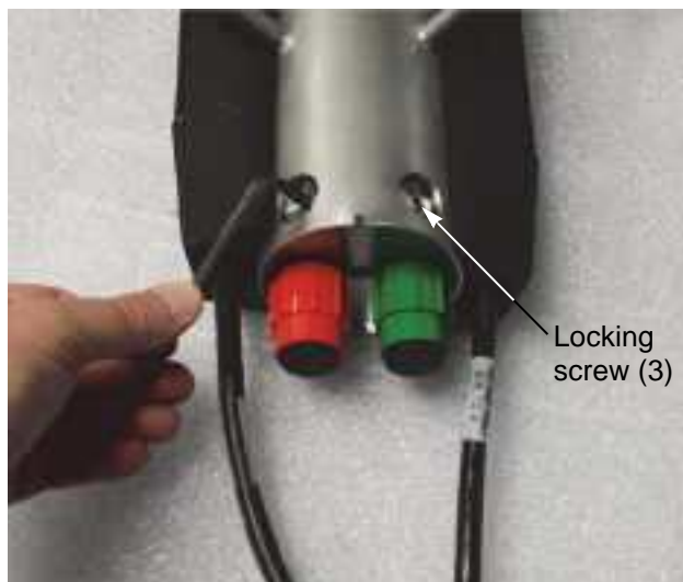
Figure 4-6: Tightening the Locking Screws in the Towfish Housing Forward End Cap
