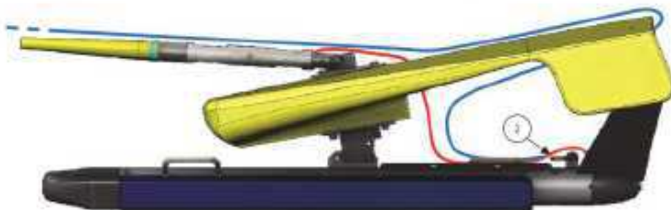
S4XXX & MA-X CONFIGURATION WITH ARMORED TOW CABLE & K-WING 2
