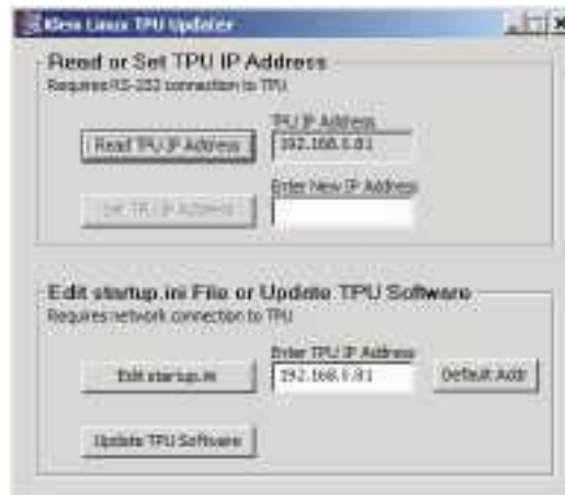
Figure C-3: The Klein Linux TPU Updater Dialog Box with Current TPU IP Address Displayed
