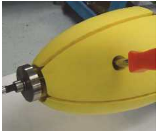
Figure 4-5: Tail Cone Being Tightened With Screwdriver and Key
