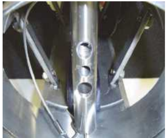
Figure 4-1: Towfish Tail with Rear Center Pin in Place
