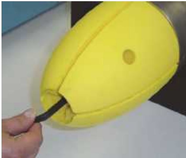
Figure 4-2: Tail Cone being Aligned and Attached to Towfish
