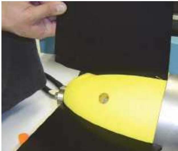
Figure 4-6: Tail Fins being Inserted into Tail Cone
