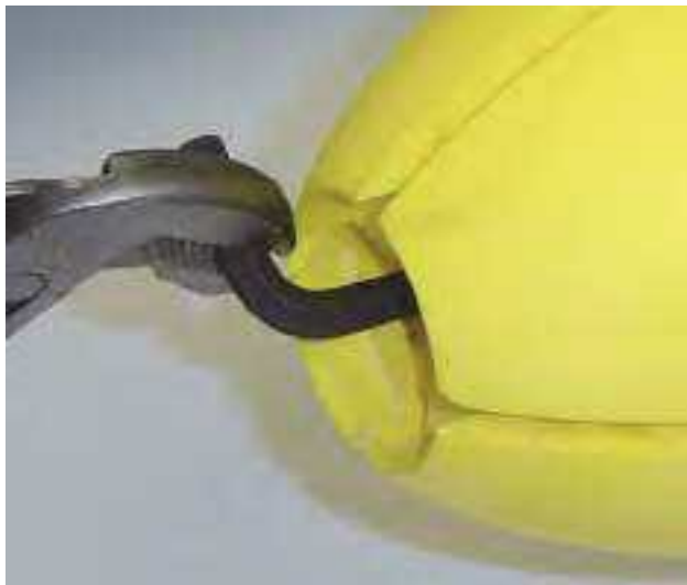
Figure 4-3: Tail Cone Being Tightened with Hex Key
